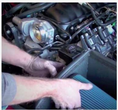
Position inlet tube and filter for best fit and tighten clamps on inlet tube and filter.
