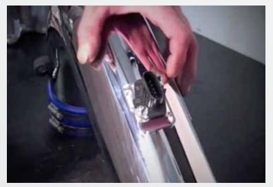
Remove mass air sensor from the stock inlet tube and install it into the aluminum mounting Block, on the BBK inlet tube with supplied screws.
