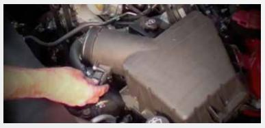
Unplug mass air sensor in inlet tube by air cleaner box.
